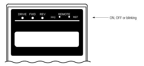
Figure 18 Operation Mode LEDs
