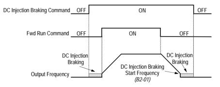
Figure 35 DC Injection Braking Contact Input Timing Diagram
