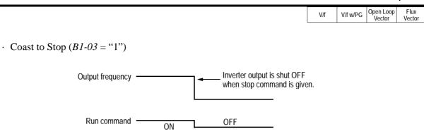
Figure 2 Stopping Method - Coast to Stop
