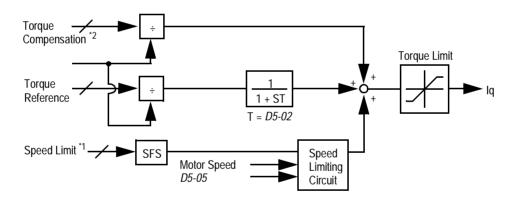
Figure 27 Torque Control Block Diagram
