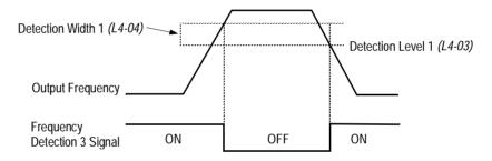
Figure 44 Frequency Detection 3 Signal Timing Diagram
