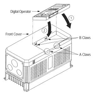
To replace the digital operator, engage the operator onto the A tabs in the direction shown by arrow 1 and then press the operator onto the B tabs in the direction shown by arrow 2, locking the digital operator into place.
