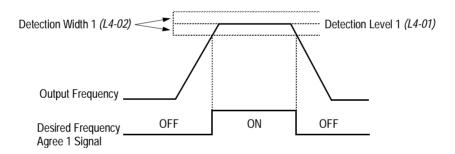
Figure 38 Desired Frequency Agree 1 Signal Timing Diagram
