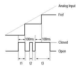
Figure 34 Sample/Hold Selection - Analog Reference
