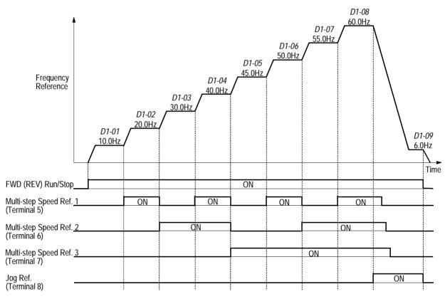
Figure 24 Multi-step Speed Operation - Timing Diagram
