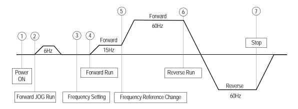
Figure 15 Operation Sequence by Digital Operator
