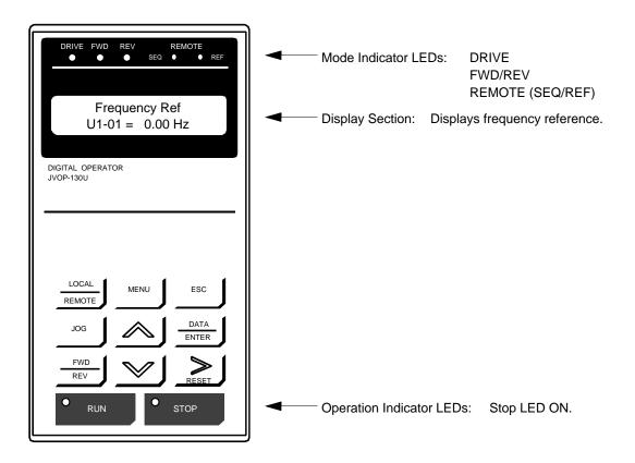
Figure 14 Digital Operator Display at Power-up
