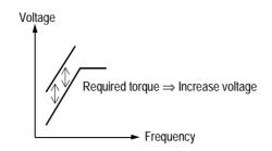
Figure 18 Torque Characteristics
