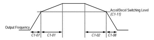
Figure 14 Accel/Decel Switching Level Adjustment
