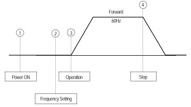
Figure 16 Operation Sequence by Control Circuit Terminal Signal
