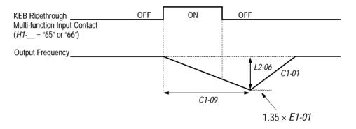
Figure 36 KEB Ridethrough Timing Diagram
