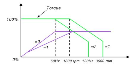
When running the motor only in the constant torque region, leave parameter C3-05 set to 0 for the best performance.
