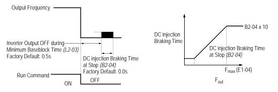
Figure 21 Stopping Method - DC Injection Braking Stop
