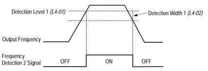
Figure 40 Frequency Detection 2 Signal Timing Diagram
