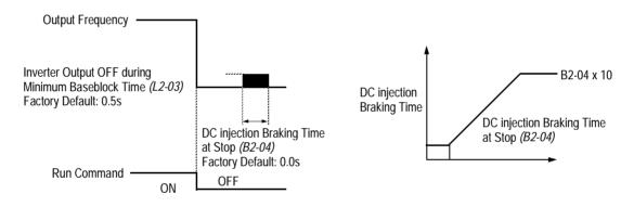
Figure 3 Stopping Method - DC Injection Braking to Stop
