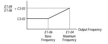
Figure 17 Slip Compensation Limit Adjustment
