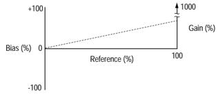
Figure 46 Analog Input Gain and Bias Adjustment
