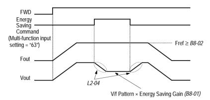
Figure 10 Timing Diagram of Energy Saving Function
