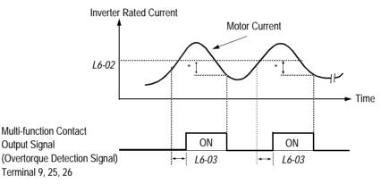
\* Release width (hysteresis) during overtorque detection is 5% of the inverter rated current level.
