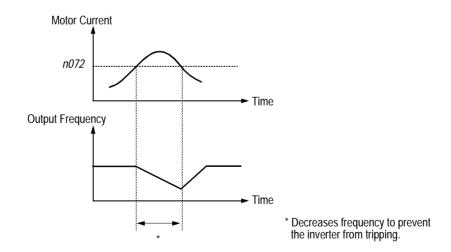
Figure 54 Stall Prevention/Current Limit During Running
