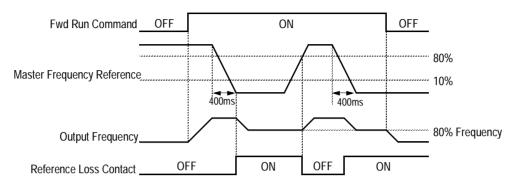
Figure 41 Reference Loss Timing Diagram
