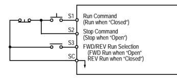
Figure 31 Terminal Function at 3-Wire Sequence Selection (H1-\_\_ = "0")
