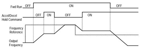
Figure 32 Accel/Decel Hold Command Timing Diagram
