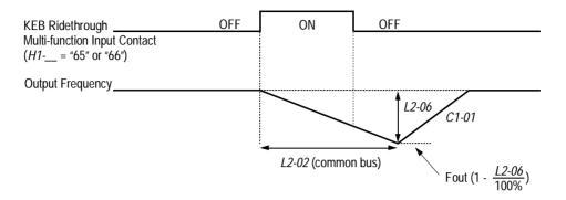
Figure 50 KEB Ridethrough Timing Diagram
