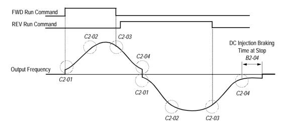
Figure 16 S-curve Characteristics - FWD/REV Operation
