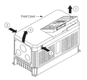
To remove the front cover, first remove the digital operator (see previous section). Then squeeze the cover on both sides in the direction shown by arrows 2 and lift the cover in the direction shown by arrow 3.
