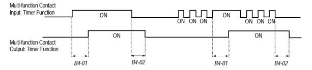
Figure 8 Timing Diagram of Timer Function
