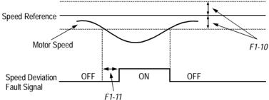
Figure 30 Overspeed Detection Timing Diagram
