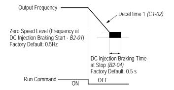
Figure 19 Stopping Method - Deceleration to Stop
