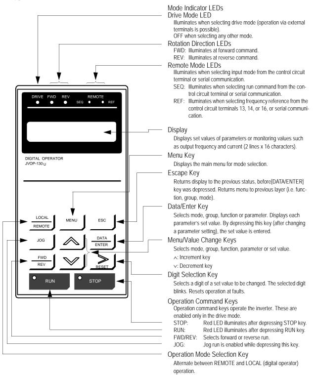
Figure 17 Digital Operator Display at Power-up
