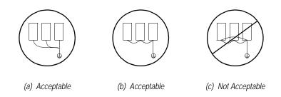
Figure 12 Grounding Example of 3 B900 Inverters
