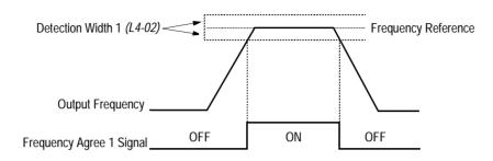
Figure 37 Frequency Agree Signal 1 Timing Diagram
