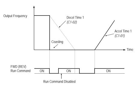
Figure 22 Stopping Method - Coast to Stop w/ Timer
