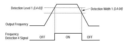
Figure 45 Frequency Detection 2 Signal Timing Diagram
