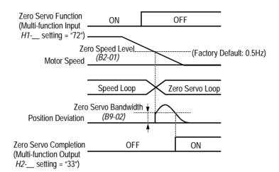
Figure 12 Timing Diagram of Zero Servo Function
