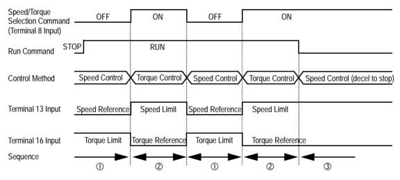
Figure 28 Speed/Torque Control Selection Timing Diagram
