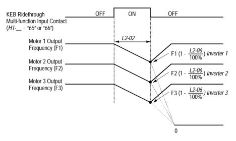
Figure 51 KEB Ridethrough - Common DC Bus Applications
