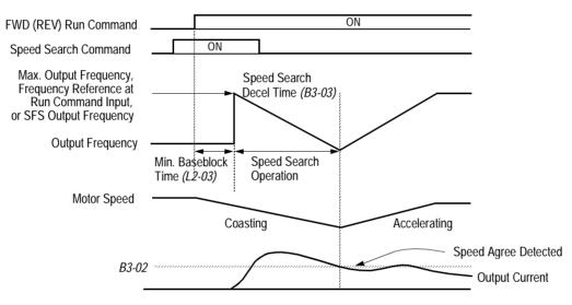
Figure 7 Search Command Input Timing Diagram
