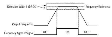
Figure 42 Frequency Agree Signal 2 Timing Diagram
