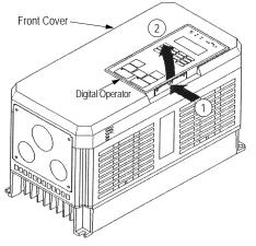
To remove the digital operator from the front cover, push the operator retaining tab in the direction shown by arrow 1 and lift the digital operator in the direction shown by arrow 2.
