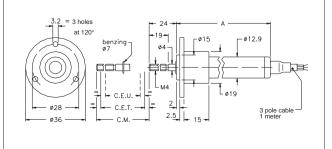
Important: all the data reported in the catalogue linearity, lifetime, temperature coefficient are valid for a sensor utilization as a ratiometric device with a max current across the cursor Ic  $\leq$  0.1  $\mu$ A.
